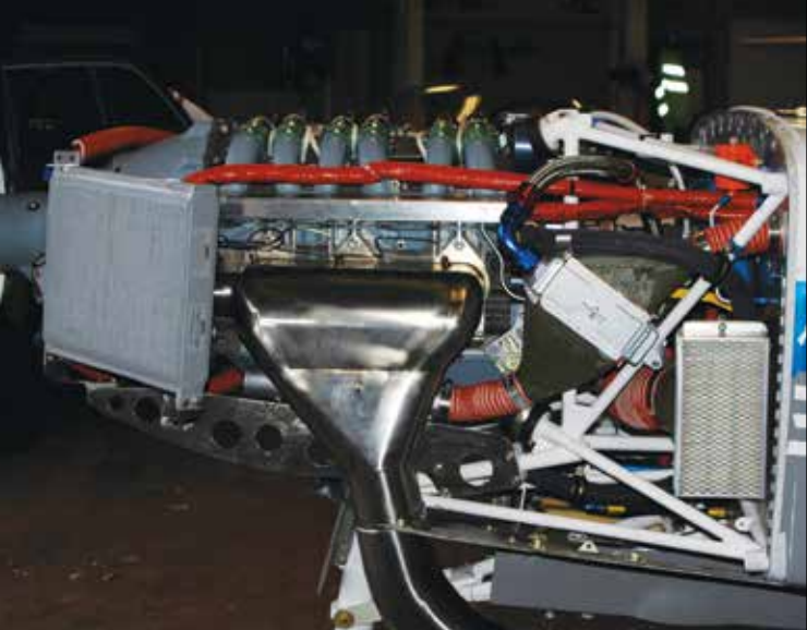
The oil cooler is mounted ahead of the exhaust collector.
