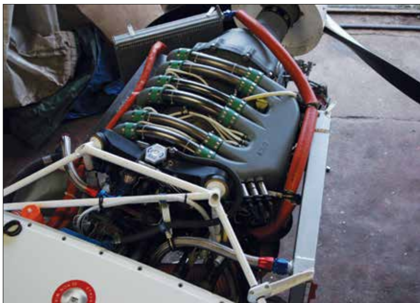
The oil cooler is mounted on the left, ahead of the engine, and the coolant radiator is on the right side.
