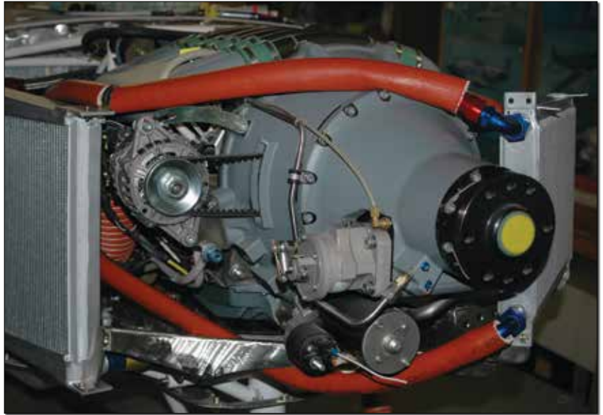
When viewed from the front, the large coolant radiator is on the left and the oil cooler is on the right.
