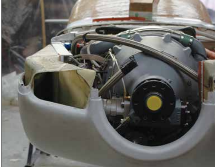
Fiberglass cooling duct for the radiator.
