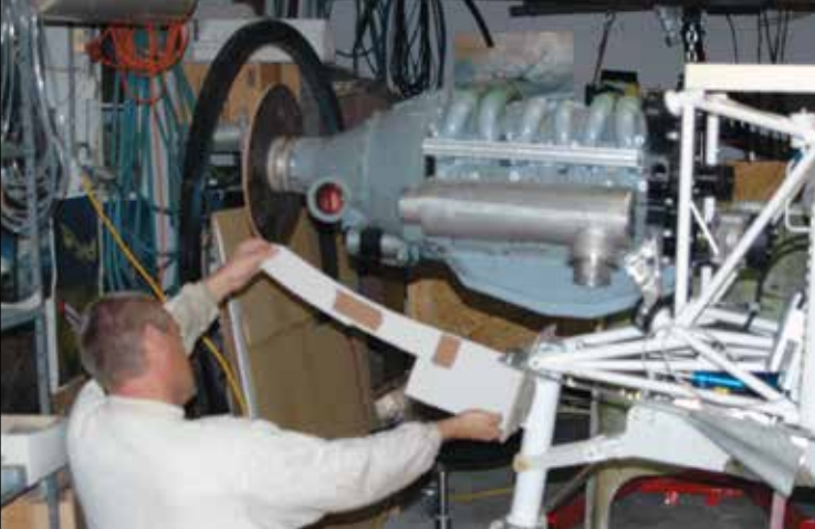
The engine mockup allowed me to design the new engine cowling.
