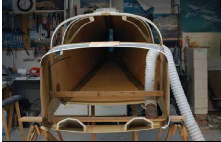
Gluing the fuselage shells together.
