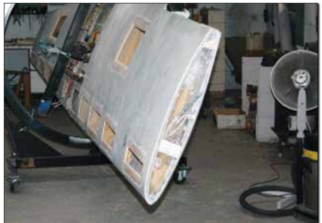
Holes for applying an ethanol-proof coating to the tanks.
