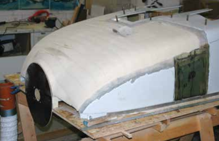
Here the lower cowling is ready for fiberglass.
