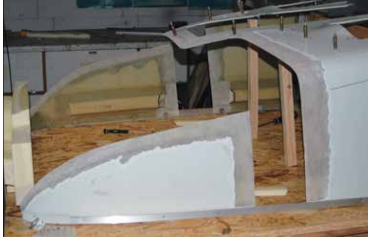
This is what I could use of the original lower cowling.
