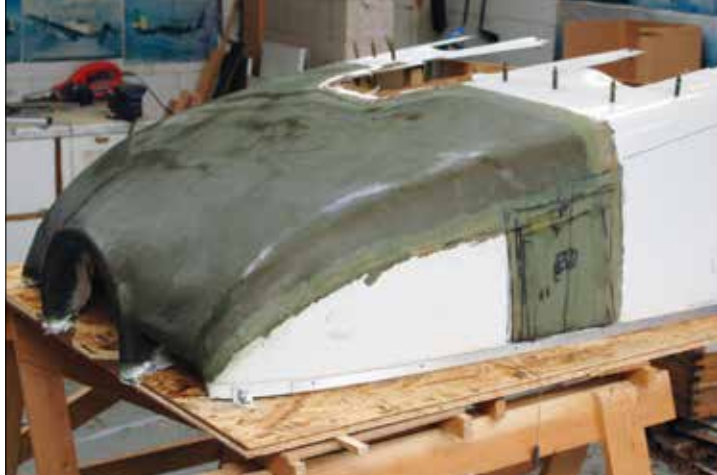
The lower cowling after adding a four-inch extension.
