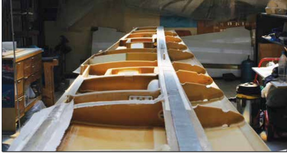
Ribs attached to the lower skins of the one-piece wing.
