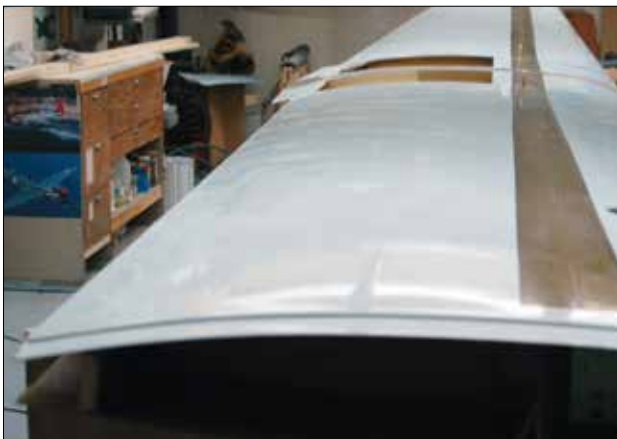
The completed one-piece-wing.
