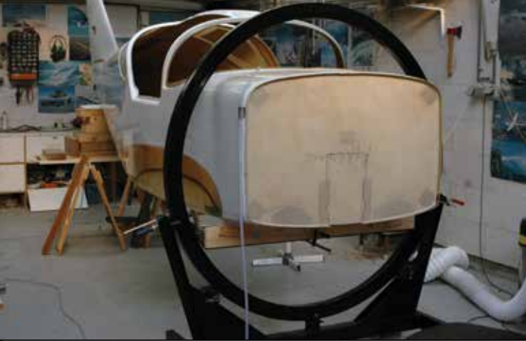
I made the ring that allowed me to fully rotate the fuselage.
